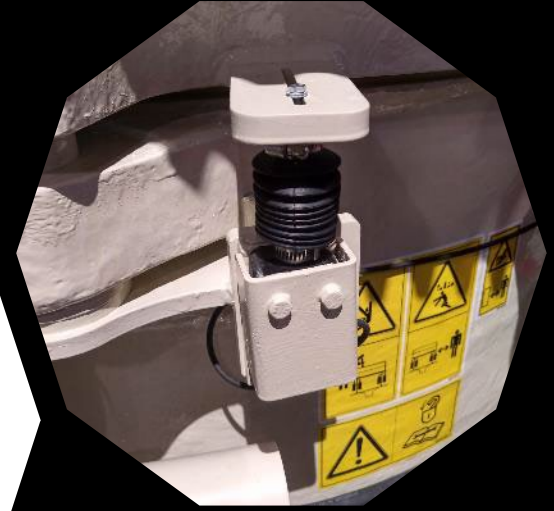
Feature: Ring bounce monitoring (with IC70C)
