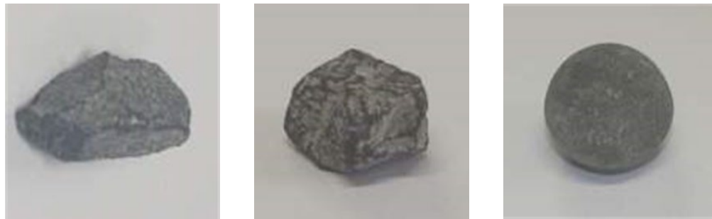
Figure 4 Aggregate shape difference; flaky, cubic and round
