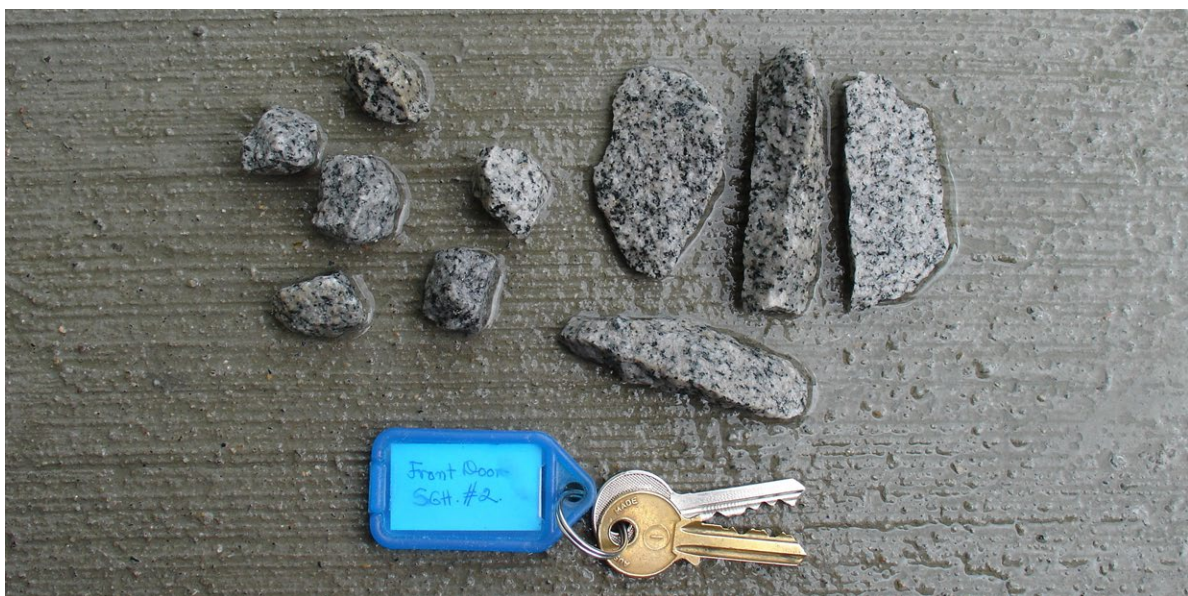
Figure 5 Flaky vs cubic shaped aggregate
