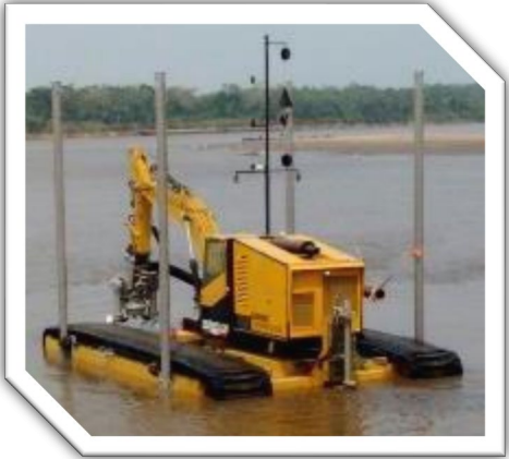
Amphibious digger, boom mounted
