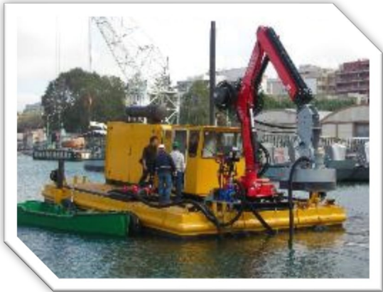
Manned dredge, boom mounted
