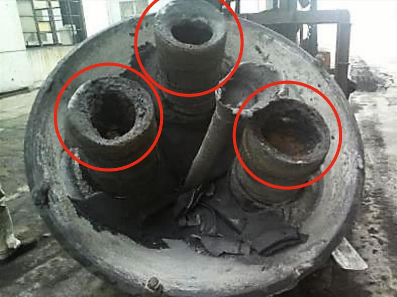
At Metso Outotec, every cast is specifically planned and simulated, and high quality is ensured by using enough risers.
