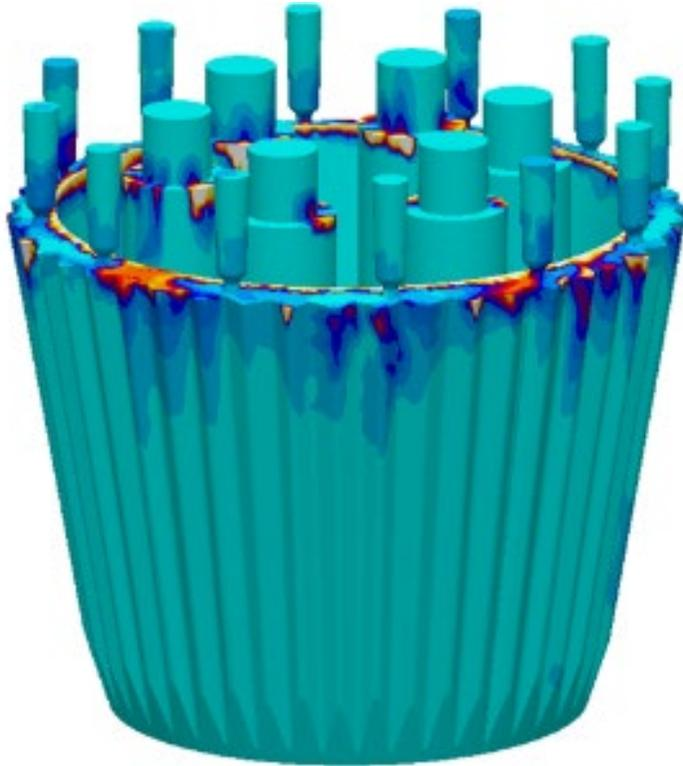
A simulation software is a standard part of our foundry method planning. It helps eliminate casting defects and ensures high quality of the final product by verifying the accuracy of the method plan.
