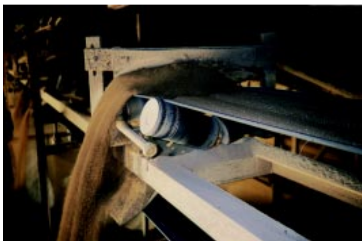
LIME BEING DROPPED INTO STORAGE
