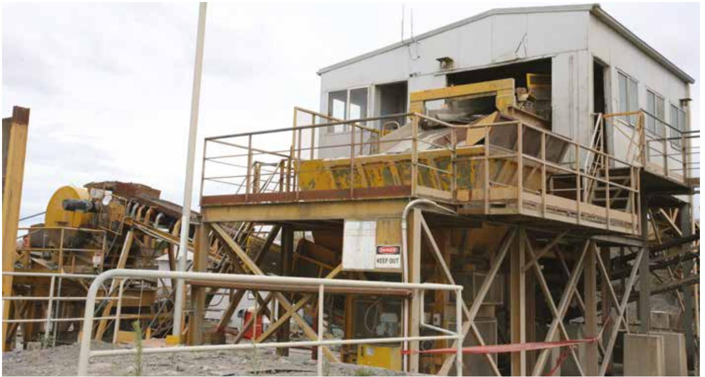
A GP200 cone crusher is the main crusher used for harder materials at one of the country's largest alluvial operations, Holcim's Hastings Quarry. Photographed in 2018.
